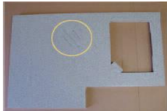
(1) Hot pot cracks
