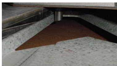
(3) Rout with 12mm(½") straight bit 25mm(1") guide
