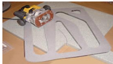
(2) Encompass damaged area
